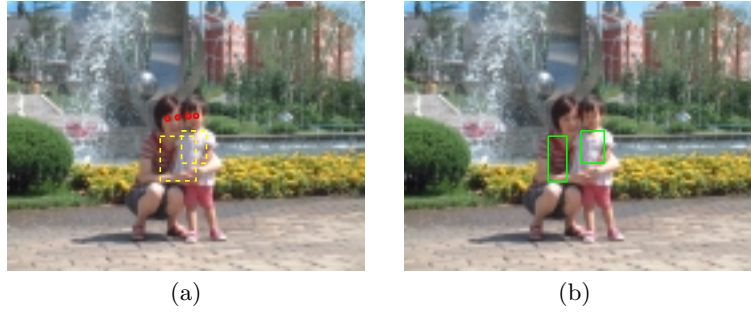
Fig. 1. (a) initial estimation from face detection (shown by the dashed yellow lines, small red circles show the eye positions); (b) refined segmentation by maximizing the difference between people (shown by the solid green lines).
